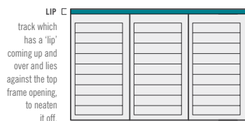
LIP Top track with lip (To neaten uneven walls, window frames, gaps etc)
